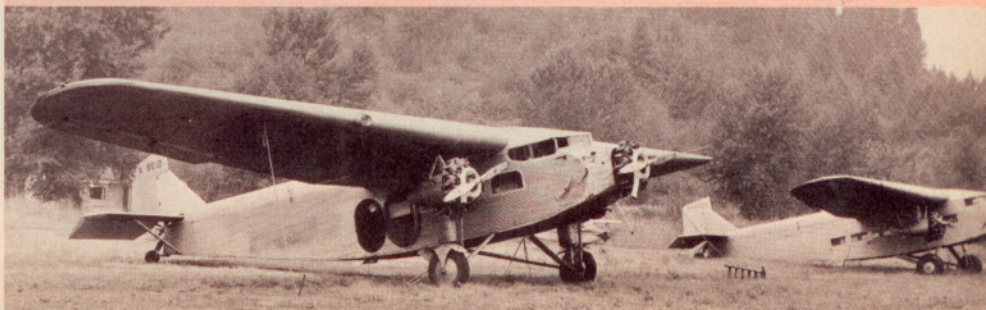
Ford's single-engine "Air Pullman" became the Tri-motor in mid-1920's. Photo shows one of the first production Tri-motors with open pilot's cockpit, half-moon windows and 200 h.p. Wright J-4 Whirlwind engines
